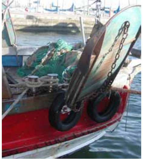
A heavy «door» (light blue) is to keep the bottom trawl net open and down to the seabed so as to flush the catch.
